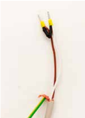
4 Green/yellow shield ground connection
