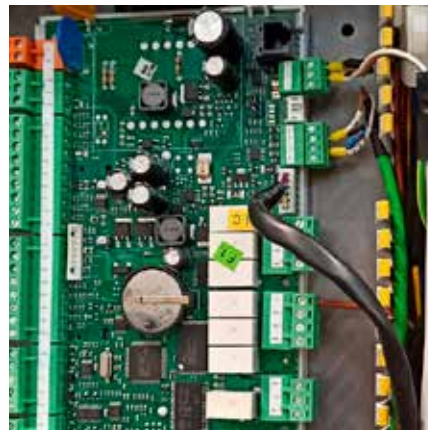
⑥a \mu PC PLAN connection
