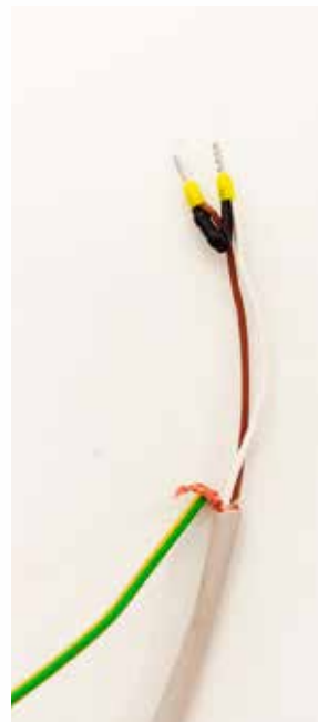
③ Green/yellow shield ground connection
