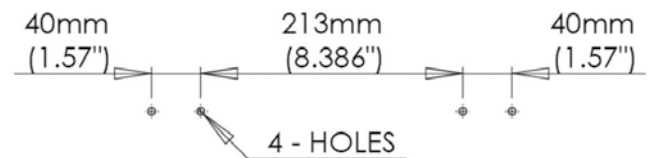
Fig P - Drilling hole template dimensions for wall mounted brackets - 3 heaters
