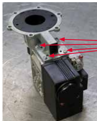
Photon 120 gas valve fixing screws
