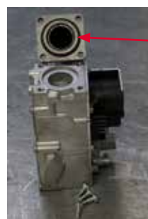
Photon 100 gas valve inlet flange assembly
