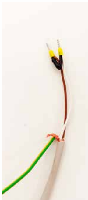
3 Green/yellow shield ground connection
