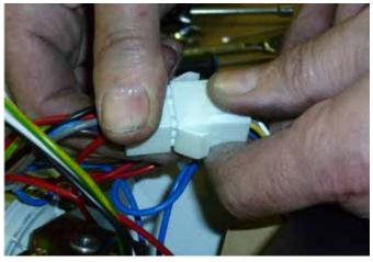
e: Disconnect ignition wire from controller (3b)
