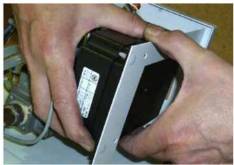
f: Release three push clips (32) from controller fixing holes.
