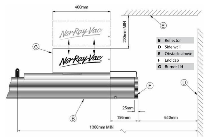
fig. 1.c Clearance for servicing - distances to obstacles above.
