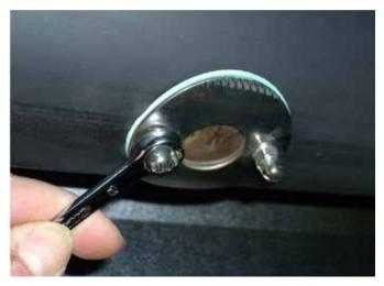
b: Unscrew dome nuts (53) remove spring washers (54). Remove sight glass cover (50), gasket (51) and mica window (52).
