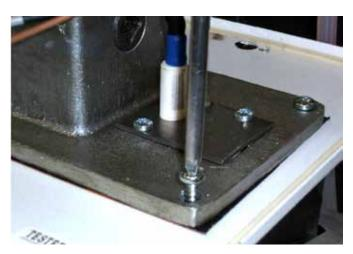
h: Lift burner clear of combustion chamber and withdraw.
