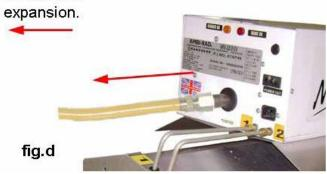
The methods shown below are unacceptable, due to undue stress on the hose & fittings.
