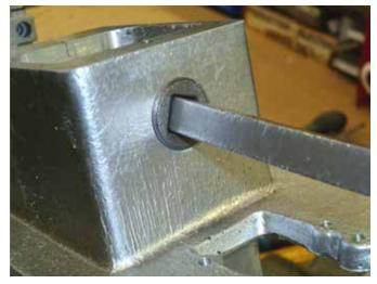
f: Unscrew brass jet (10) inside mixing chamber using 8mm allen key and withdraw through 1/2in BSP hole.
