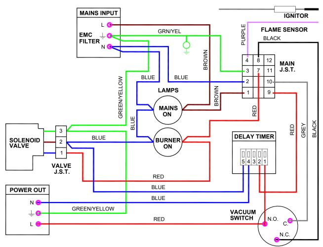
Figure 4.d. NRV M internal wiring diagram - In-line Burner (IL)
