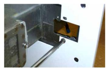
g: Remove valve bracket set screws (36) from the underside of burner base plate.
