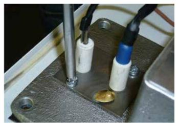
f: Carefully withdraw electrode assembly from burner - noting electrode orientation.
