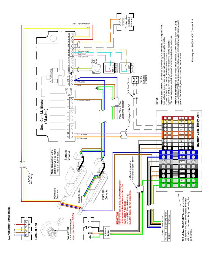
Figure 4.s. NRV M System Schematic interconnecting wiring. BH300 three phase fans.
