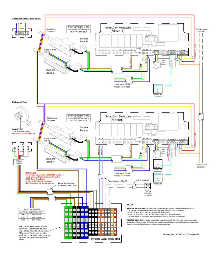
Figure 4.p. NRV M System Schematic interconnecting wiring. BH300 three phase fans. Modulating controlled by SmartCom3 via three phase inverter panel. (single zone shown)
