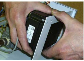
f: Release three push clips (32) from controller fixing holes.
