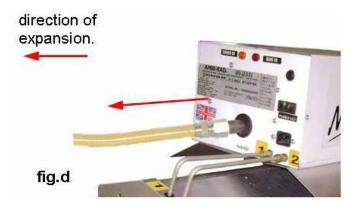
The methods shown below are unacceptable, due to undue stress on the hose & fittings.
