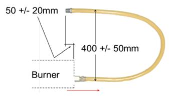
The correct installation as shown below will allow for approx 100mm of movement due to expansion
