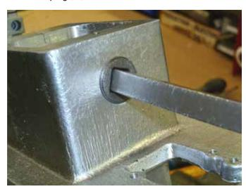
f: Unscrew brass jet (10) inside mixing chamber using 8mm allen key and withdraw through 1/2in BSP hole.
