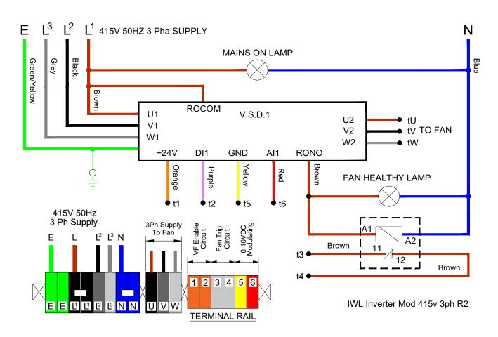
Figure 4.m. NRV M System Schematic interconnecting wiring. B80, B160 and B300 three phase fans. Modulating controlled by SmartCom3 via single phase inverter panel. (single zone shown)
