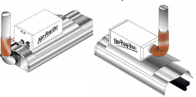
fig 5.e. Burner Ducted Air Inlet Connection
