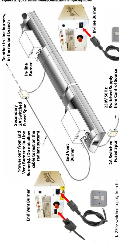
3. Connect a mains lead from the secondary
