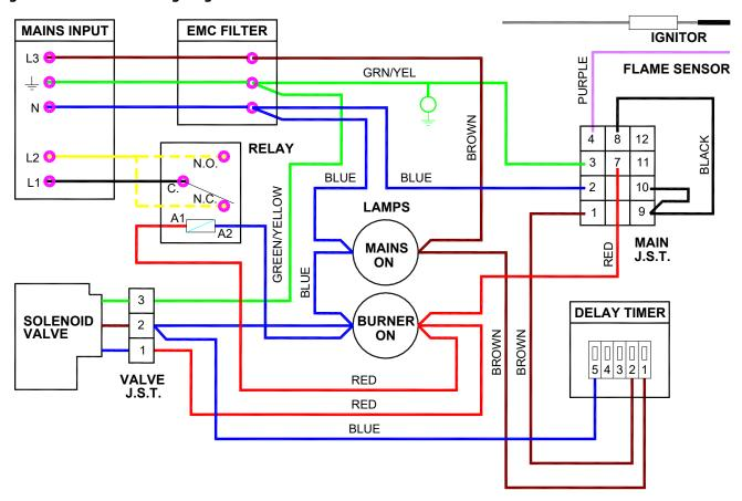
Figure 4.g. M internal wiring diagram - End Vent Burner c/w 3 way solenoid valve
