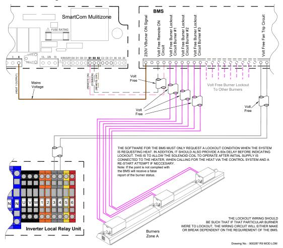
Figure 4.v. Additional wiring for NRV M zonal burner lockout
