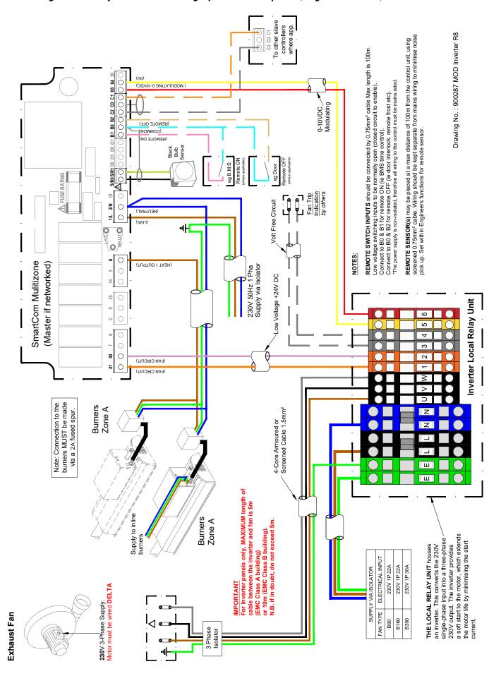
Figure 4.n. NRV M System Schematic interconnecting wiring. B80, B160 and B300 three phase fans. Modulating controlled by SmartCom3 and zonal branch dampers via single phase inverter panel. (1 zone shown)
