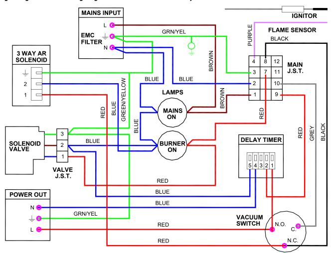
Figure 4.h. M internal wiring diagram - End Vent Burner c/w 3 way solenoid valve & N/O or N/C VF Lockout contacts
