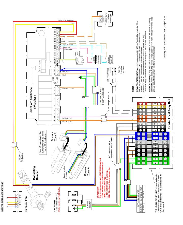
Figure 4.t. Additional wiring for NRV M individual burner lockout
