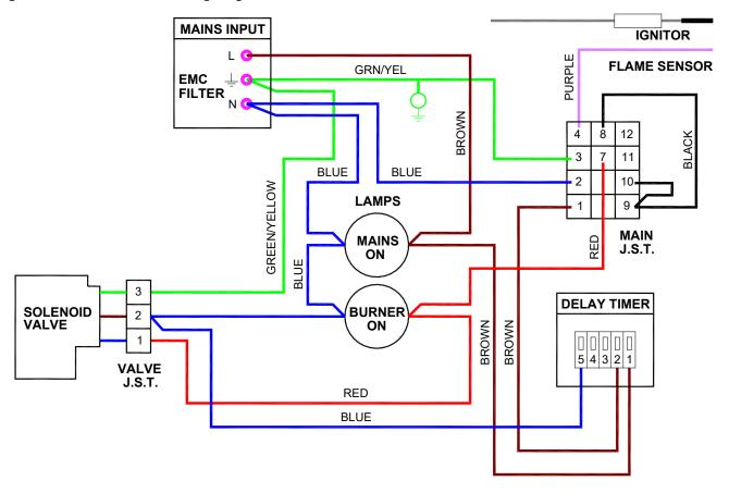
Figure 4.e. M internal wiring diagram - End Vent Burner c/w N/O or N/C volt free Lockout contacts
