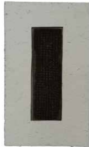
Burner with face insulation in place
