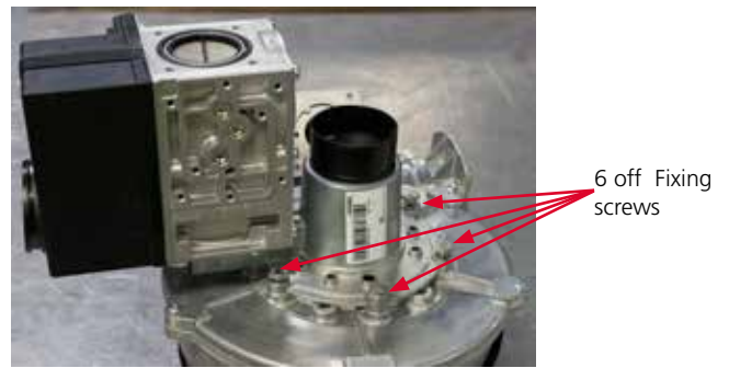
Photon 120 remove combustion fan to reveal gas valve fixing screws
