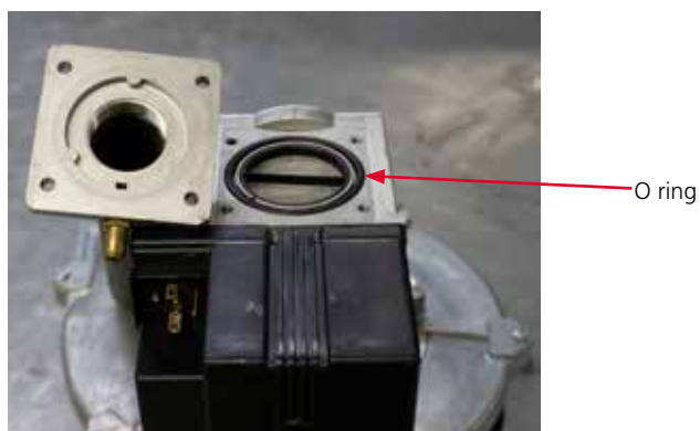
Photon 120 gas valve inlet flange assembly
