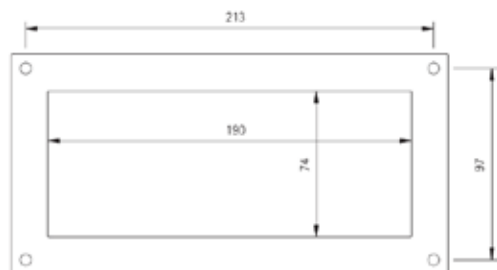
Figure 4c. Type 'O' Fan Outlet Dimensions
