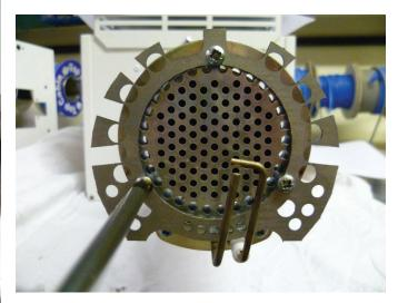
Step 2 The pepper pot burner head can be replaced if necessary ensuring the 5 holes on the outer ring are aligned alongside the probes.
