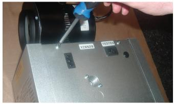
Step 8 Open the two side doors and remove the rear plate assembly.
