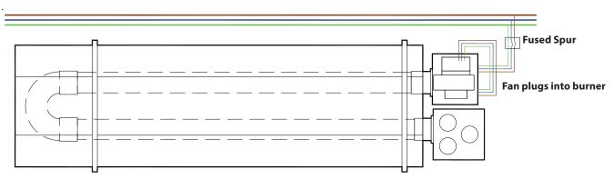
fig.5a VSX Internal Burner Wiring Diagram (Optional Webber solenoid shown in dotted)
