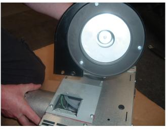
Step 4 Remove the fan orifice plate and spigot.
