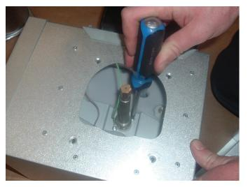
Step 7 Turning the housing over, remove the four screws holding the rear burner plate in position.
