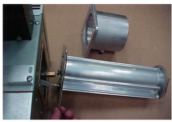
Step 2 The burner head assembly can be removed by firstly disconnecting the silicon tube from the pressure test point, the earth cable and withdrawing the probe lead once disconnected the from the controller.
