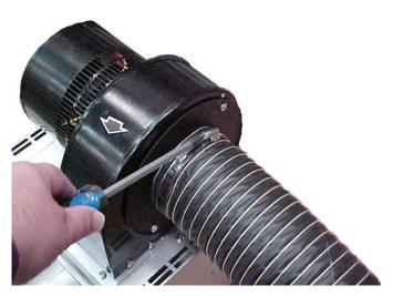
Step 5 Slacken the set screw on the burner support casting. Remove the burner from the radiant tube and position the burner in a safe area to prevent the burner or components attached to the burner from falling to the ground.
