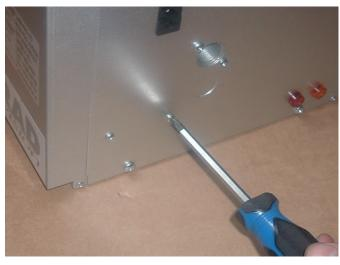
Step 3 The air pressure switch can now be removed.
