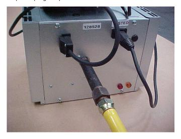
Step 3 Detach the gas supply as shown below, taking care to support the burner connection.
