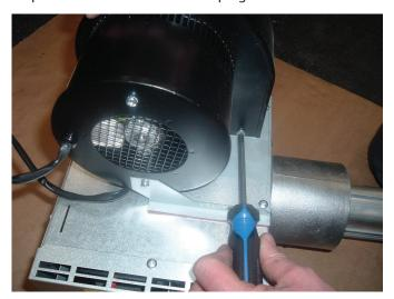
Step 3 The combustion fan can now be detached.
