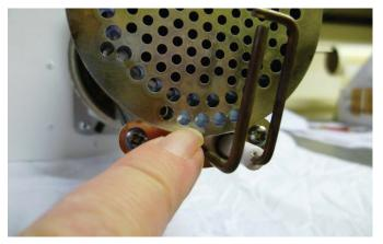
Step 3 The condition of the ignitor assembly can be checked for deterioration. However, we advise replacement at each service to ensure continued reliability.
