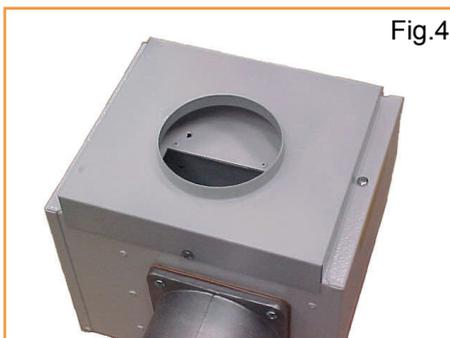
c) Fit one of the hose clips to the end of the flexible coupler. Slide the flexible coupler over the spigot on the ducted air lid and tighten the hose clip as shown in fig.5.
