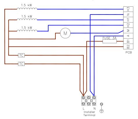
Figure 4. MINI 1000SE6 6.0kW Wireless internal wiring
