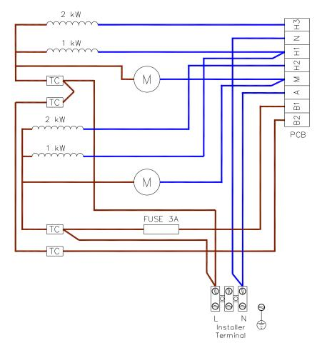
Figure 5. MINI 600SE3 3.0kW internal wiring.
