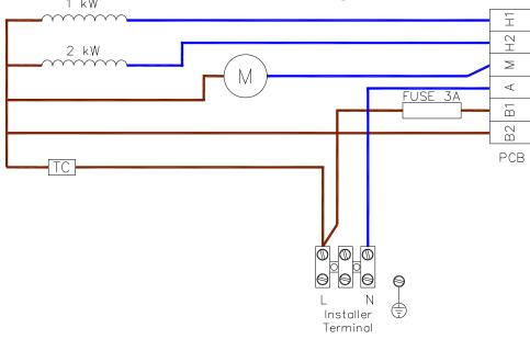
Figure 3. MINI 800SE4-5 4.5kW Wireless internal wiring
