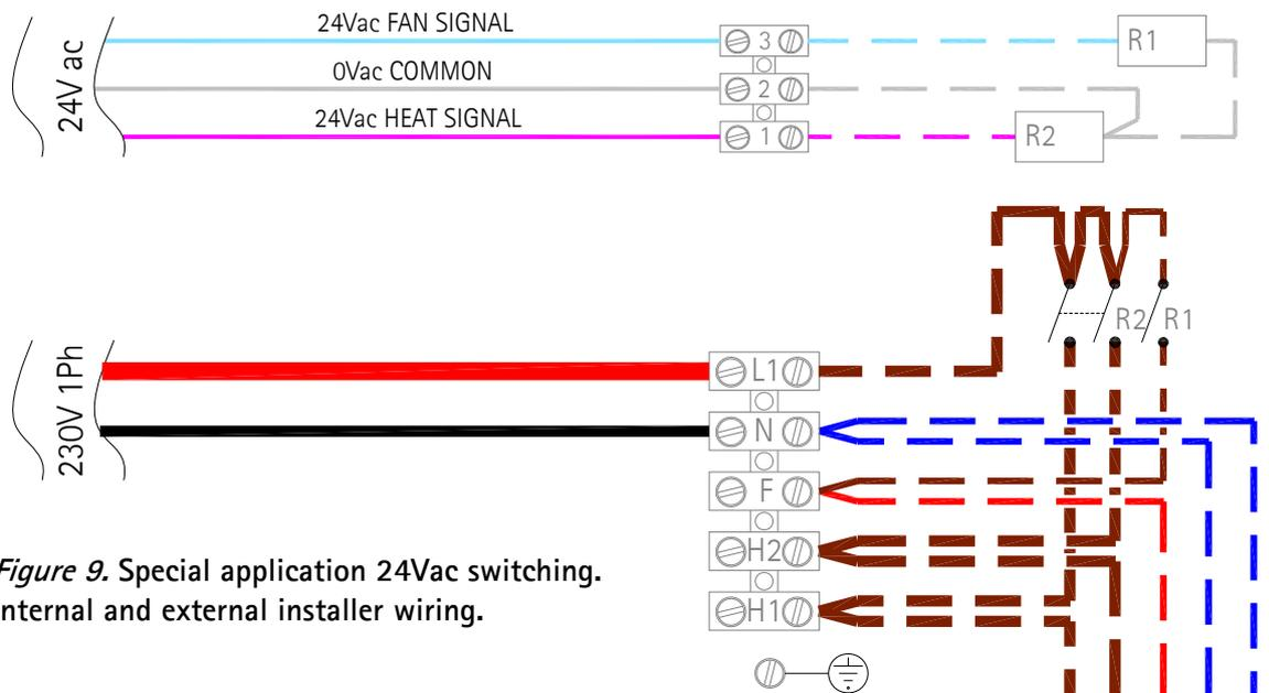
Figure 9. Special application 24Vac switching. Internal and external installer wiring.
