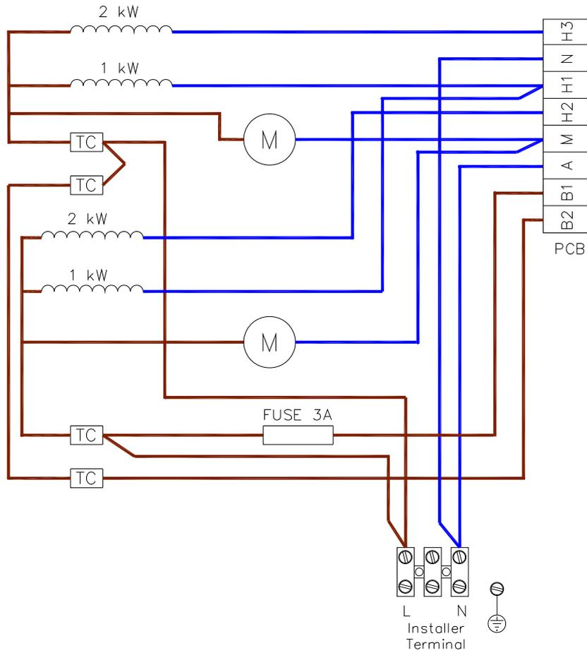
**Figure 5. MINI 600SE3 3.0kW internal wiring.**
