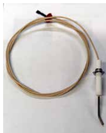
Flame probe Length of probe = 46.55mm overall 32.95mm to angle 13.79 mm angle to tip Tip deflection away from 0° = 27°
