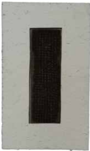
Burner with face insulation in place
