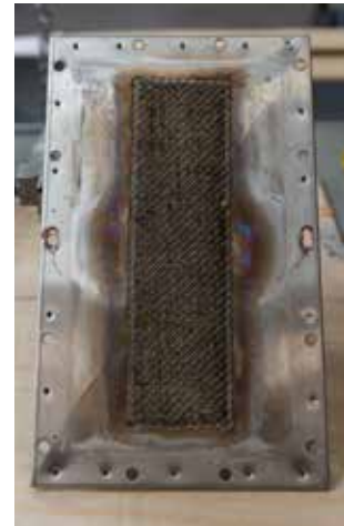
Burner with face insulation removed
