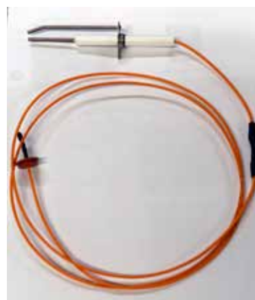
Spark probe Length of probe = 78.5mm long probe 42.3mm short probe 3.5±0.5 mm gap between probes Angle of probe = 20°
