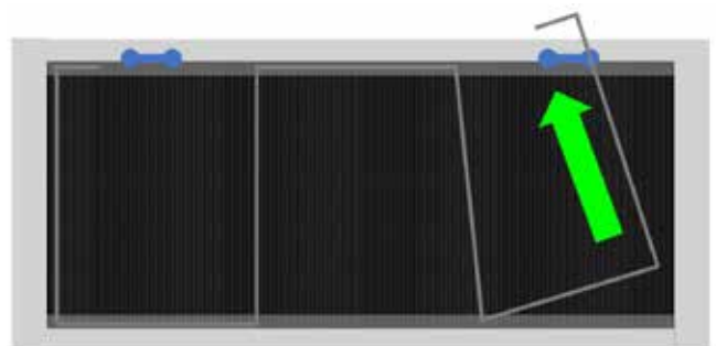
Figure 27.1 GS removing the inlet foam retaining clip
