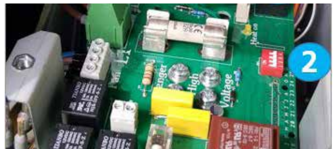
Figure 23 DIP switch position
