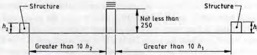
Fig 11 Flat roof, where the flue outlet is more than 10 heights ( h ) away from all structures
