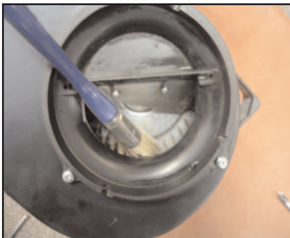
Open access door. Remove 2 screws.
