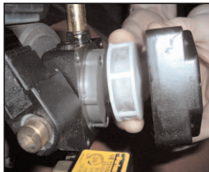
Check and clean pump filter.
