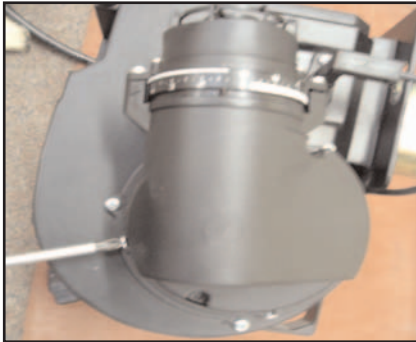
Clean impellers internally.
