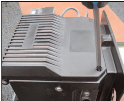
Open access door. Remove 2 screws.
