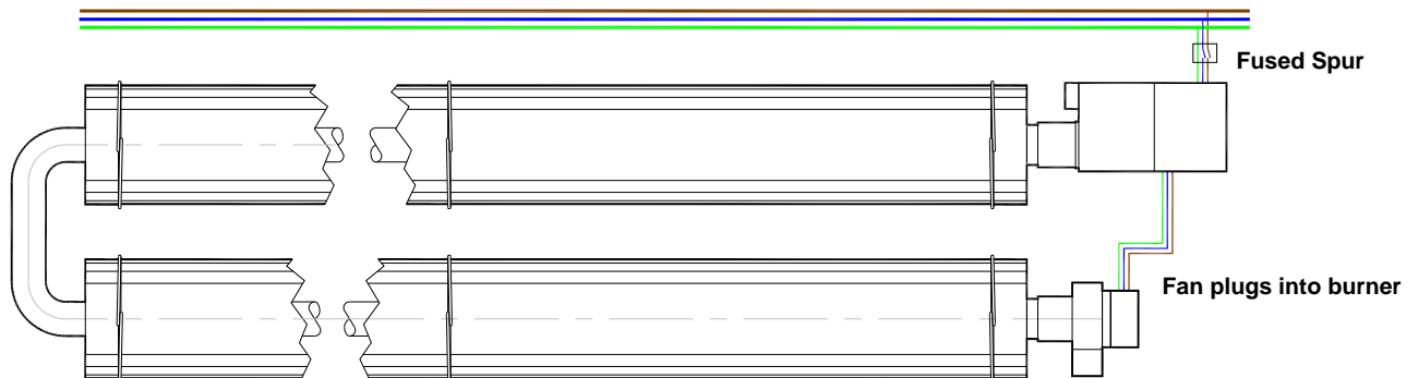
Figure 7.a Typical ARUT/AREUT Wiring Connections
